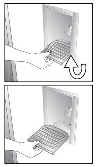
Make sure that the parts removed (if any) during cleaning are properly attached to their original places. Otherwise, water leakage may occur.
